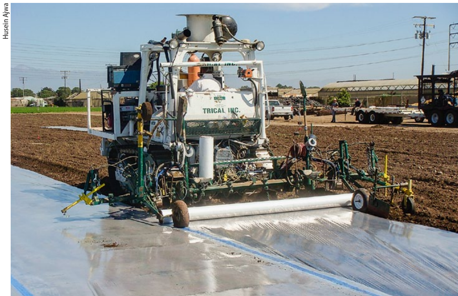
Data from the Oxnard trial indicate that a longer tarp-covering period than the standard 5 days is needed to reduce emissions associated with tarp cutting. Above, broadcast shank fumigation under TIF, Oxnard, Ventura County, September 2009.
