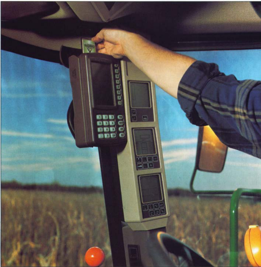
Inside the combine's cab, the operator utilizes a data card to transfer data from the monitor to the computer.
