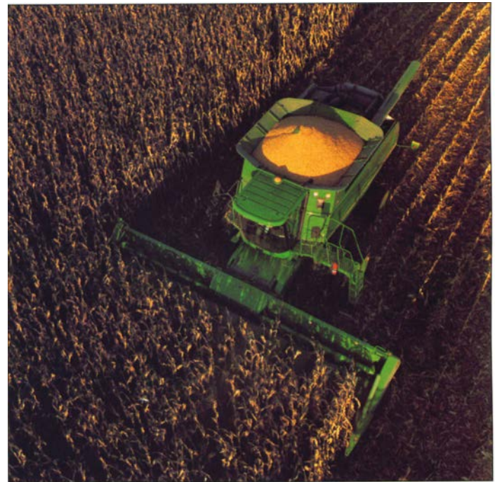
A yield monitor-equipped combine harvests a corn field.
