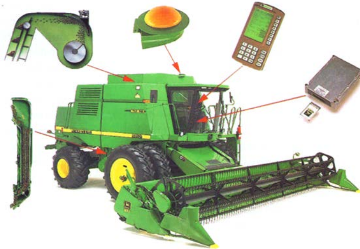
Components of a combine-mounted yield-monitoring system. Clockwise from left, Motion sensor, yield monitor, global positioning system, yield-monitor display and data-recording device. Photo composite courtesy of John Deere Company.
