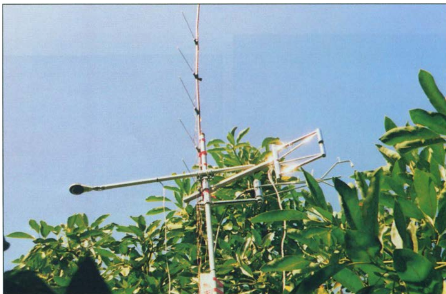
Energy balance measurements over an avocado orchard near Camarillo to estimate evapotranspiration.
