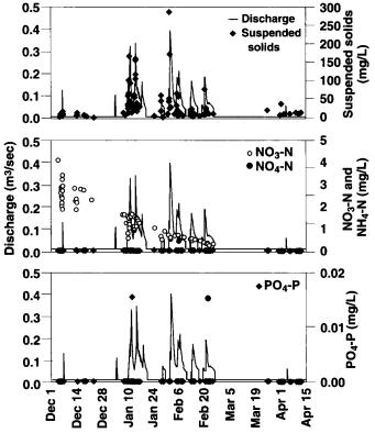
Fig. 2. Stream flow and constituent concentrations from SFREC Watershed 2 for the period Dec. 1, 1997 through April 15, 1998. (cfs =  $35.31 \times m^3$ / sec).
