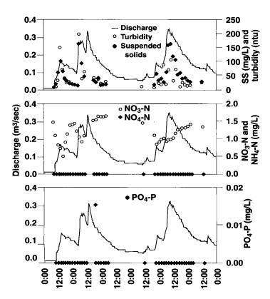
Fig. 1. Stream flow and constituent concentrations from SFREC Watershed 2 for the period of Jan. 11-16, 1998. (cfs =  $35.31 \times m^3$ / sec).
