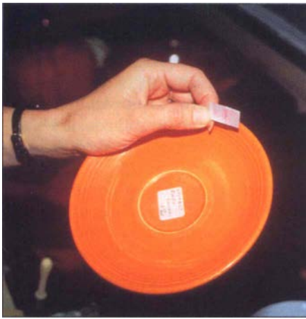
▲ The UC Quick Lead Test indicates by color change, from clear to pink, that lead has leached out of this saucer.
