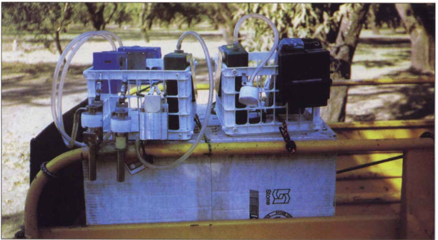
▲ Dust samples were collected on filters held in plastic cassettes connected to battery-powered vacuum pumps. The two samplers on the left are connected to size-selective cyclones that allow sampling of respirable dust. The sampler on the right has no cyclone and measures total dust.
