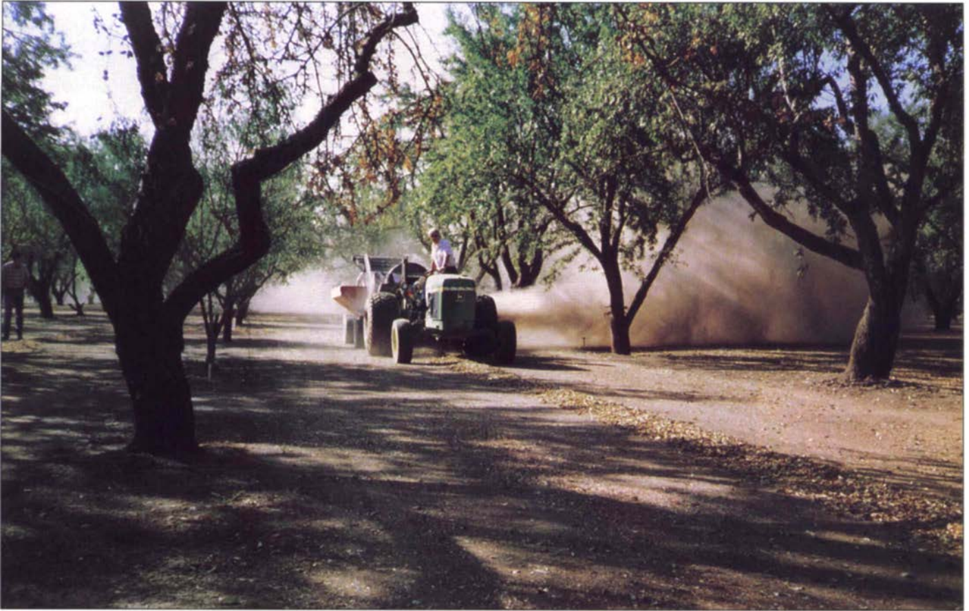
Modifications to the almond harvester allowed about two-thirds more of the windrow debris to drop to the orchard floor. In a conventional harvester, all the debris passes through the discharge fan and disperses in the air.
