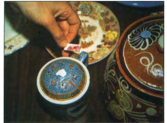
UC's 20-minute lead test uses citric acid to determine the presence of leachable lead in pottery.
