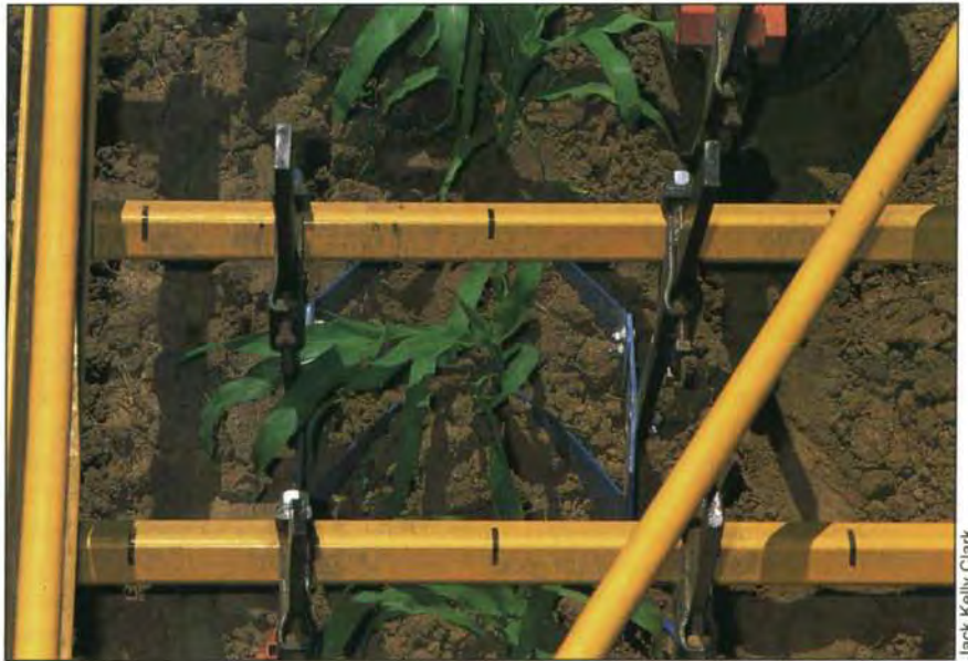
An in-row cultivator uproots weeds in the organic corn plots. The torsion rods loosen soil in the crop row, dislodging small weeds without injury to the deep-rooted corn crop.
