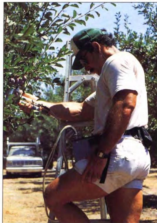
Dave Goldhamer uses a steady-state porometer to measure leaf stomatal conductance, an indicator of CO<sub>2</sub> assimilation.
