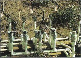
Organic fertilizers were mixed in the black tank (*left*), and then injected by pump into the drip system. Control valves and pressure gauges (*above*) were used to monitor and control emitter performance. The systems tested five different types of drip emitter; one is shown below.
