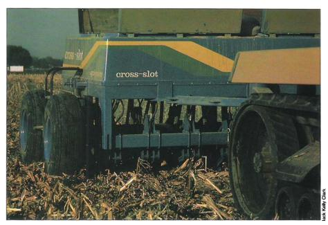
No-till drill shown above is used to plant small grains into surface stubble without plowing, a sustainable agriculture technique which reduces soil erosion and saves time and energy.
