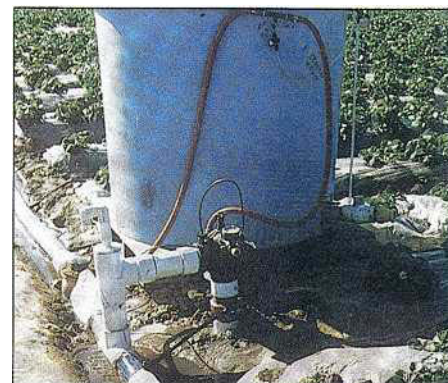
This apparatus injects an experimental polymer into drip lines, inhibiting the buildup of line-clogging sediments.
