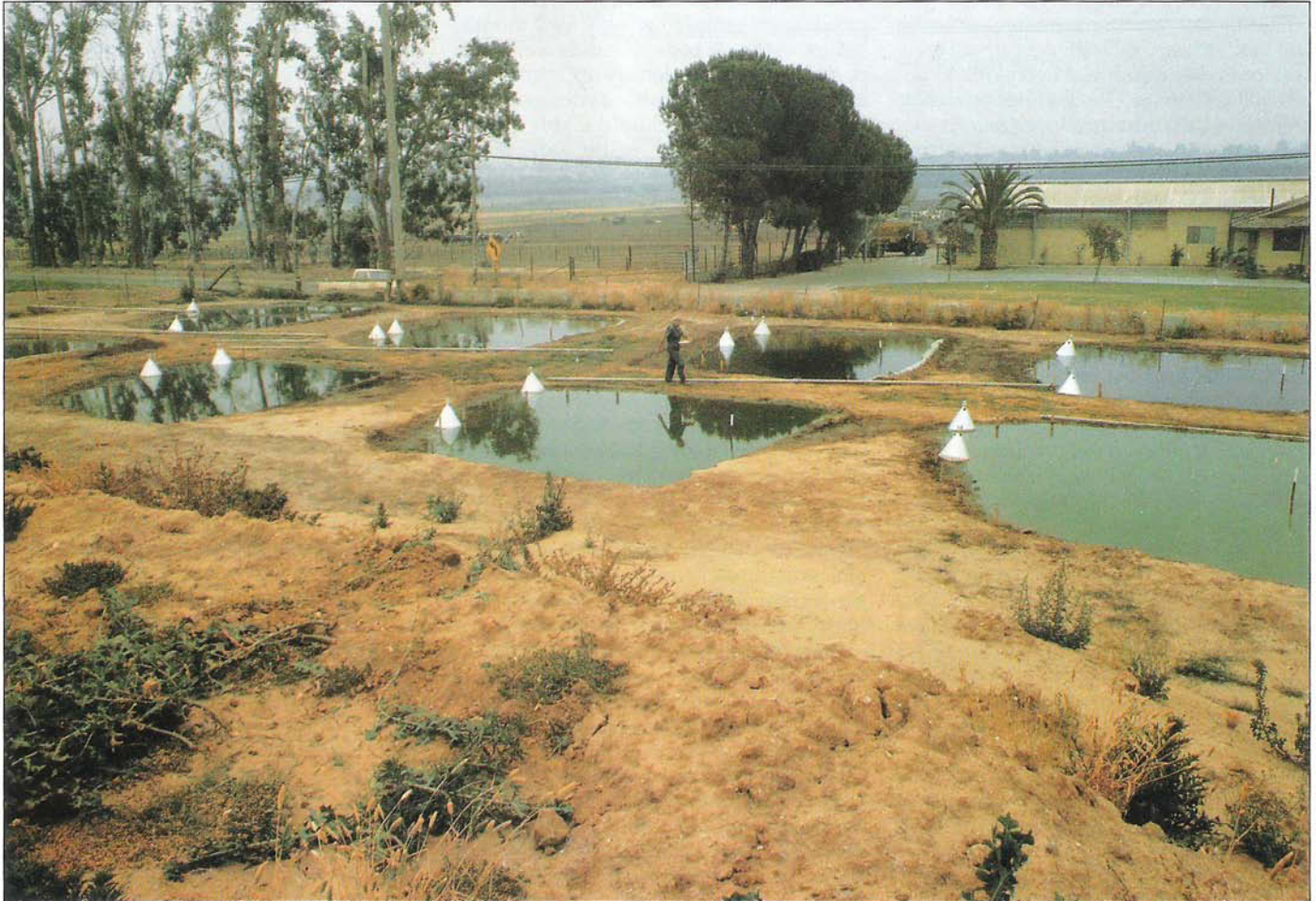
Experimental dairy wastewater ponds were used to study effects of manure loading and changes in water level on populations of the Culicoides gnats that spread bluetongue virus of cattle and sheep. The white cones are aluminum emergence traps used to collect adult gnats.
