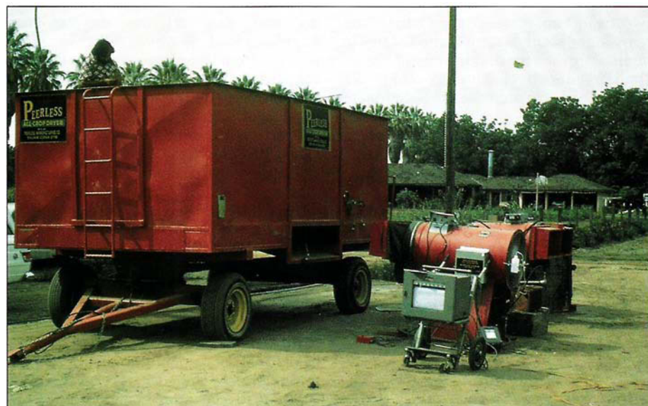
Trailer dryer is supplied with heated air from a portable fan/burner assembly. The air is directed to the nuts through a screen-covered air plenum in the bottom of the trailer.
