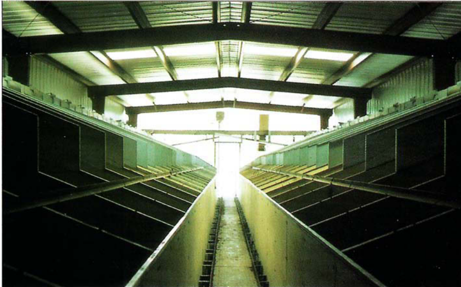
Typical fixed-bin walnut dehydrator. Doors under each bin regulate the flow of heated air through a sloped screen floor in the bin.
