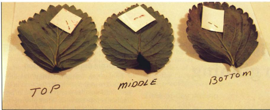
Efficiency of growers' homemade spray rigs was tested by stapling 1-inch-square dye cards to leaves in top, middle, and lower leaves of strawberry plants, and measuring coverage. None of the rigs provided adequate coverage for good pest control.
