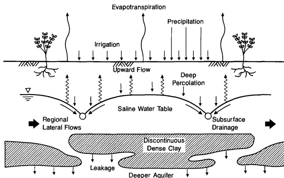
Fig. 1. Cross-section of a hypothetical tile-drained field with a shallow water table, showing water pathways into and out of the crop root zone.
