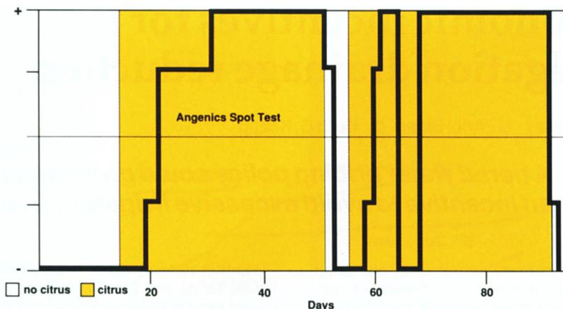
Fig. 1. Angenics Spot Test for penicillin showed false positive readings shortly after citrus pulp feeding began and returned to normal after citrus feeding ended. Other quick assay tests and the official Food and Drug Administration disc assay showed negative readings throughout the trial.
