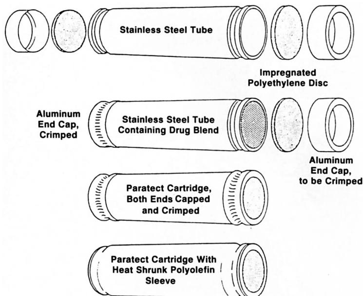
The stainless steel tube contains the deworming medication in an inert polyethylene glycol carrier, which is released through permeable polyethylene diffusion discs at each end. The entire device is enclosed in a heat-shrunk polyolefin sleeve.
