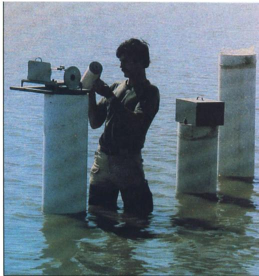
Infiltrimeters (left) were installed in Kings County evaporation pond to estimate seepage. Rainfall, evaporation, drainage flows, and changes in pond water levels (here being checked by co-author Blake McCullough-Sanden) were also measured.
