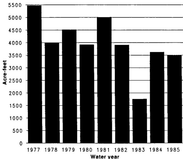
Fig. 1. Estimated groundwater flow in the study reach for the water years 1977-85, using data from a variety of water agencies. The estimates are based on a model incorporating "flow tubes" simulating hydraulic gradients.
