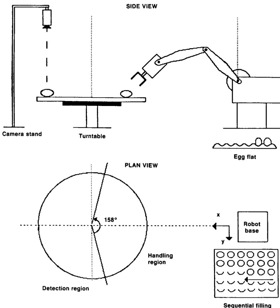
Fig. 2. Laboratory model physical layout.
