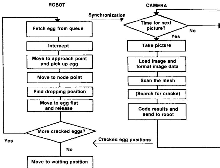
Fig. 1. Candling system block diagram.
