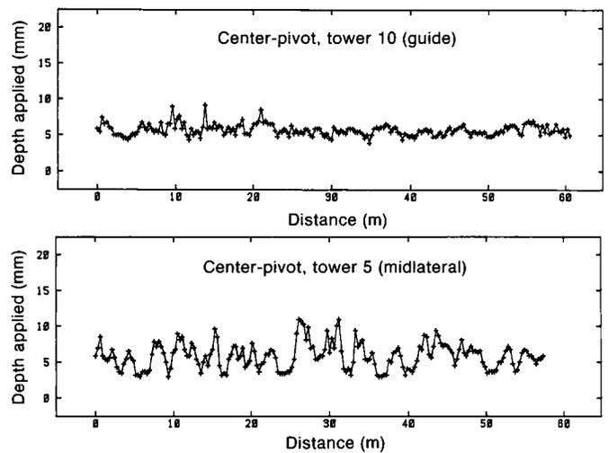
Fig. 4. Center-pivot machine showed little variability near the guide tower but repeating peaks and valleys near the midlateral.
