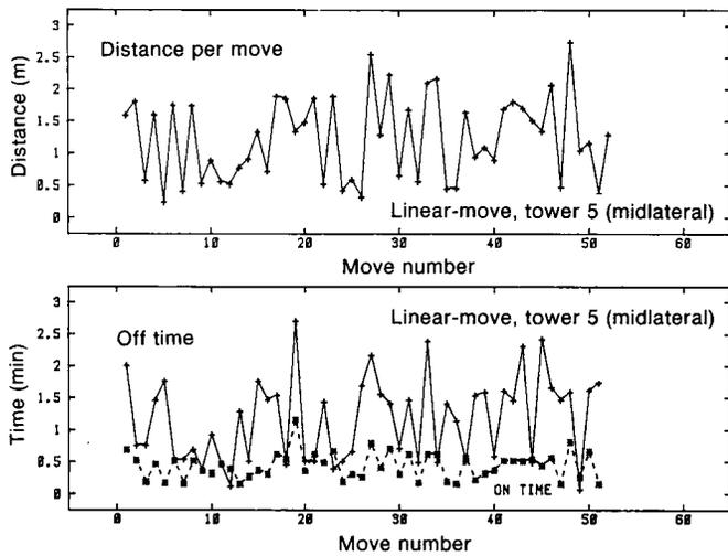
Fig. 3. Unlike pattern in fig. 2, movement of the midlateral tower of the linear-move machine was very irregular.
