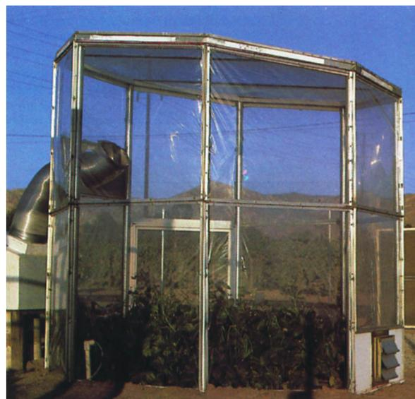
**Regulating the proportions of filtered and unfiltered air in individual octagonal closed-top chambers permitted varying concentrations of atmospheric pollutants.**
