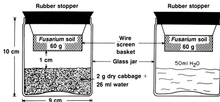
Fig. 2. The fungicidal effects of gases from dried cabbage residues are illustrated in an experiment in which infested field soil is suspended in air above the preparation in a tightly stoppered glass jar. The treatment eliminated *Fusarium* propagules. In control jar at right, containing plain water, there was no effect on the organism.
