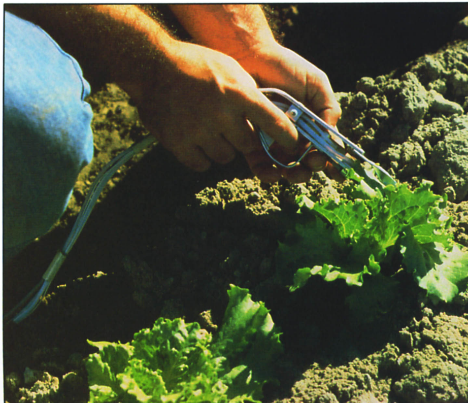
Dual isotope porometer developed by plant physiologists at U.C., Riverside, simultaneously measures effects of insecticides on lettuce photosynthesis and transpiration.
