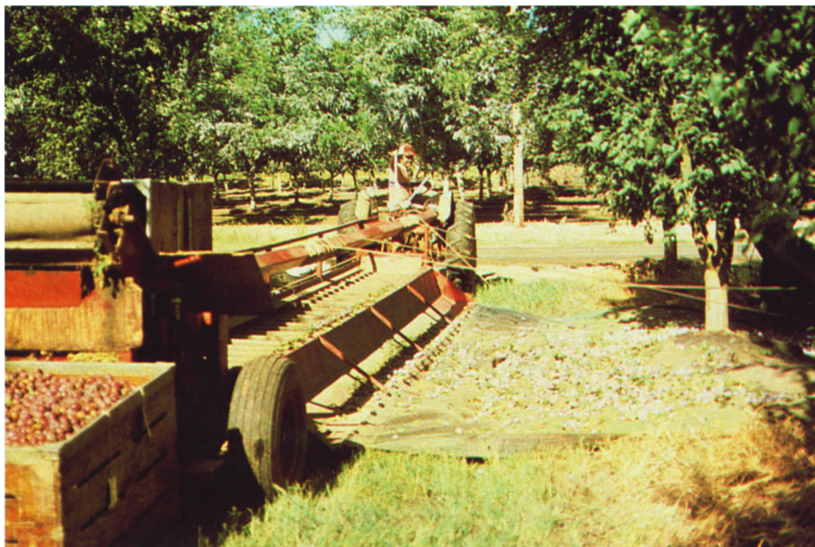
Bins used with this mechanical harvester are specially vented for fast cooling of prunes for cold storage.
