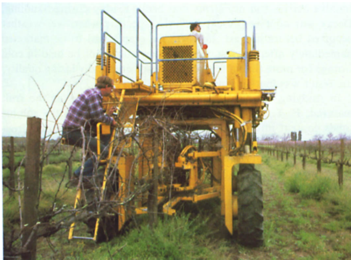
Pre-pruning vines with a modified mechanical grape harvester reduced yields of most varieties in U. C. tests. More sophisticated commercial machines facilitate pruning, but require follow-up by hand pruners.
