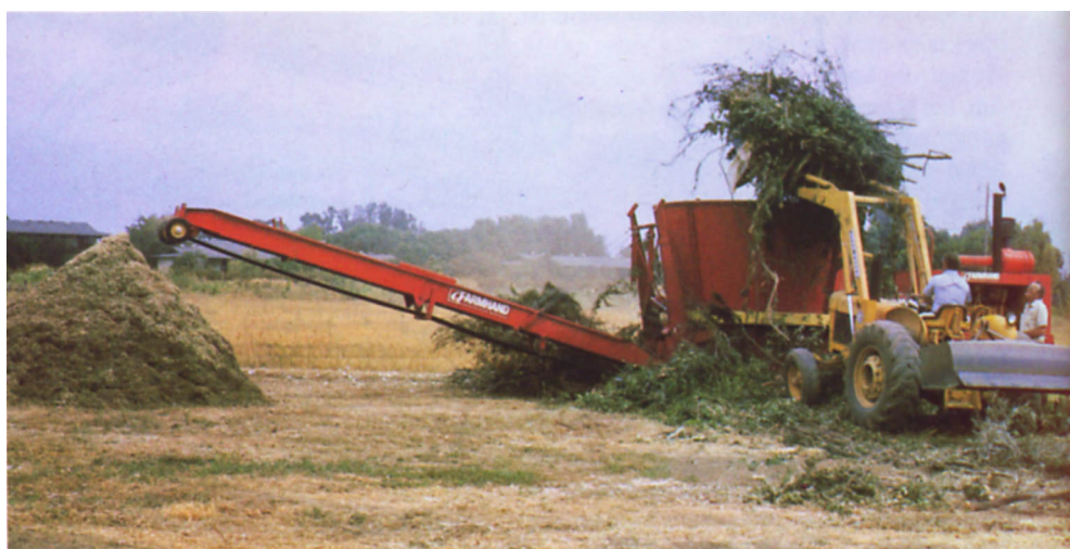
Right: Tub grinder, originally designed for hay and straw, shows promise in preparing orchard prunings, forest slash, and brush for alcohol production.
