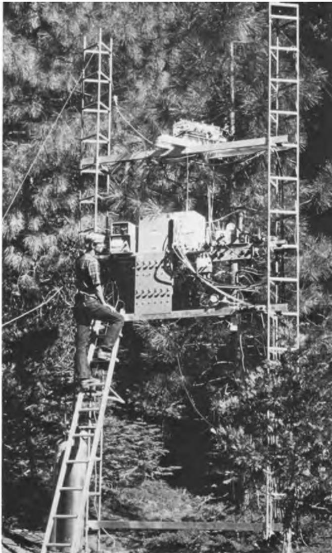
To measure photosynthesis, respiration, and transpiration in the field, a cuvette for measuring gas exchange is attached to a series of branches. Underneath the cuvette is a rack bearing analytical equipment for monitoring physiological processes.
