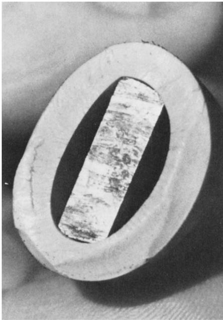
End of artificial teat used to simulate on-and-off flow of cow's teat under pulsated vacuum.
