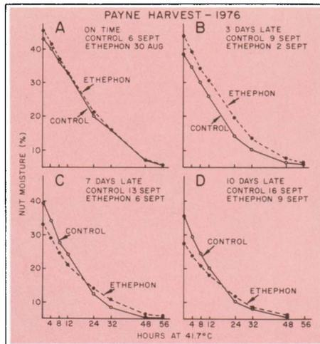
Fig. 3. Drying rate of 'Payne' walnuts at 107° F (41.7°C). (A) Harvest on time; (B) harvest 3 days late; (C) harvest 7 days late; and (D) harvest 10 days late.
