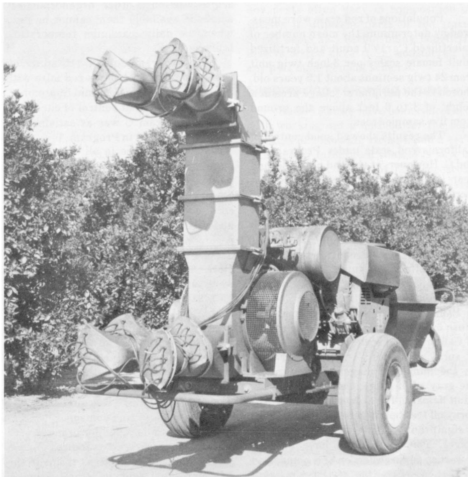
Low-volume sprayer with two discharge heads positioned at two heights on an air tower. Improved spray distribution in citrus tree top areas results in better control of red scale and red mite, key pests in an integrated control program.
