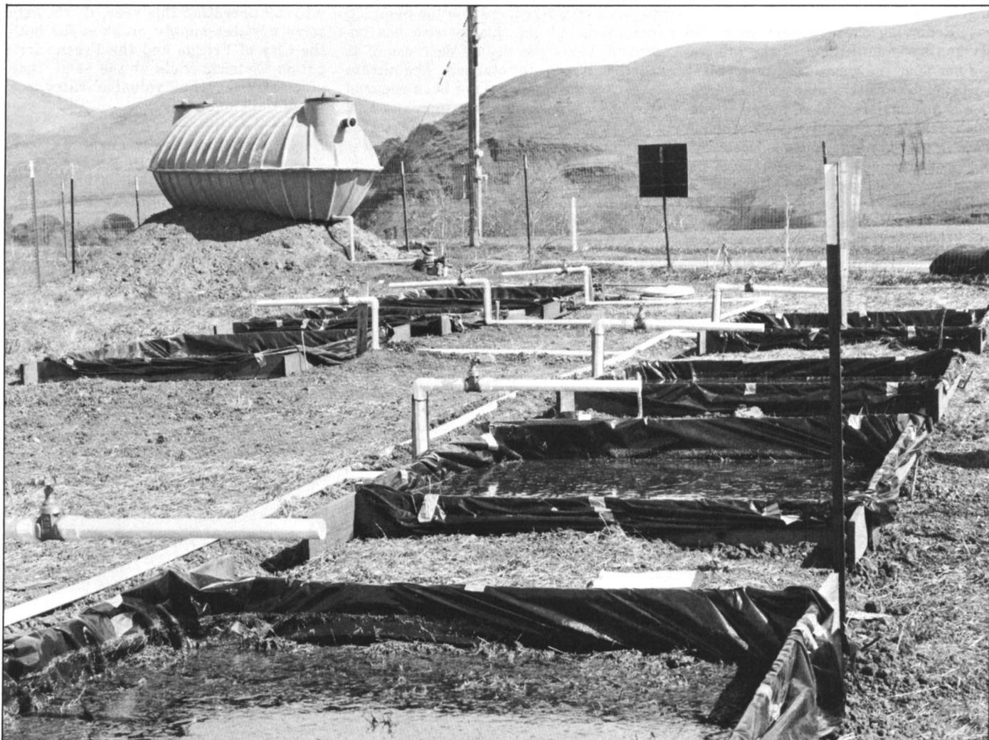
View of water percolation basins on Diablo clay soil. Fiberglass septic tank in background served as storage tank for effluent water.
