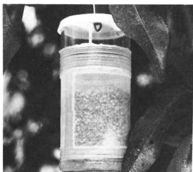
Fig. 1. Standard 25-dram navel orangeworm egg trap placed in almond tree. Note space above bait, which allows air movement through windows.
