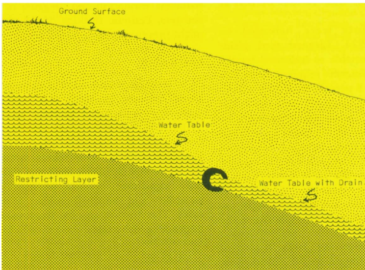
Fig. 5. Water table receding after drainage installation.
