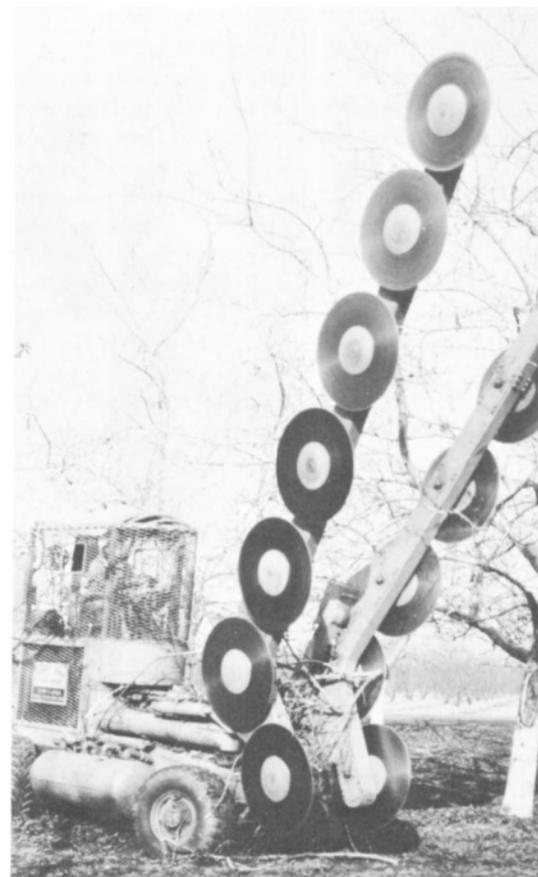
Walnut hedging machine used in these Tulare County trial featured seven circular saw blades mounted vertically on two booms, allowing trimming from either side of the row without turning around.
