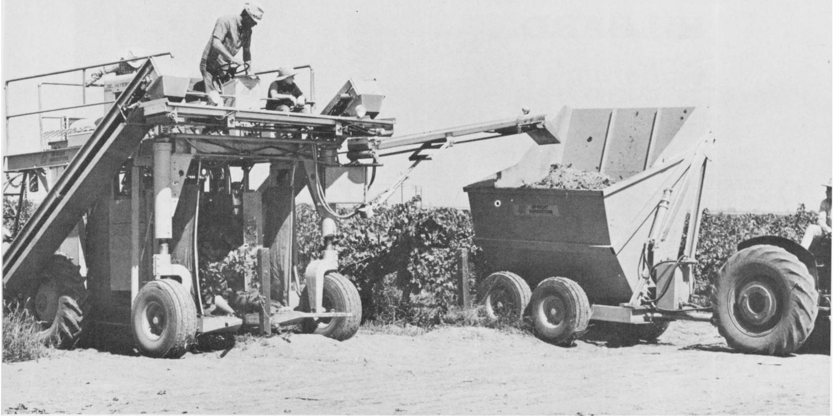
Wine grape harvesting equipment includes the grape harvester, a 5-ton self-dumping gondola, and a 40 to 60 hp tractor.
