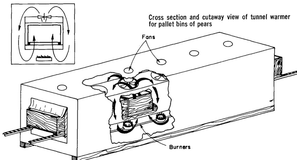
Cross section and cutaway view of tunnel warmer for pallet bins of pears
