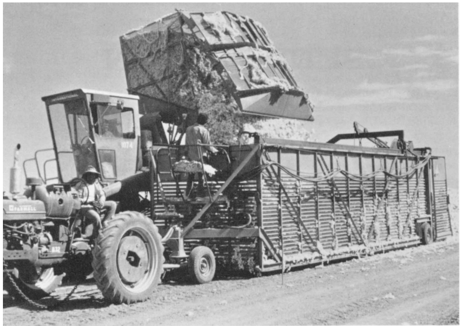
A cotton picker is shown dumping into a grower-built ricker which uses a hydraulic powered roller-compactor.
