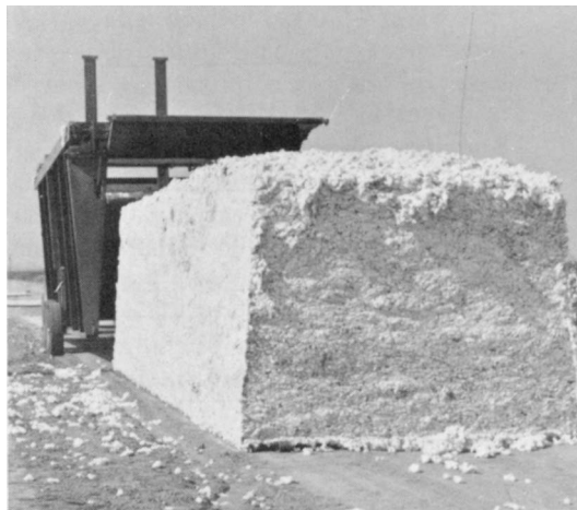
Rear view of a 24-ft module builder pulling off of a newly completed cotton module.
