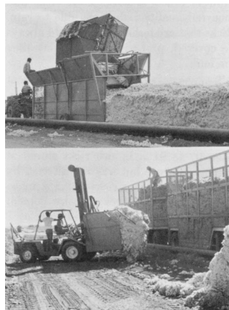
A cotton picker, top photo (and cover), is shown dumping into a Rosebud ricker. This ricker has a hydraulic ram operated compactor. Forklift and loader attachment in bottom photo is loading ricked cotton into special highway trailers for long-distance transport to a gin.
