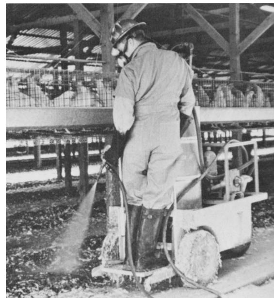
Spray unit mounted on battery-powered cart for insecticide applications inside a poultry house.
