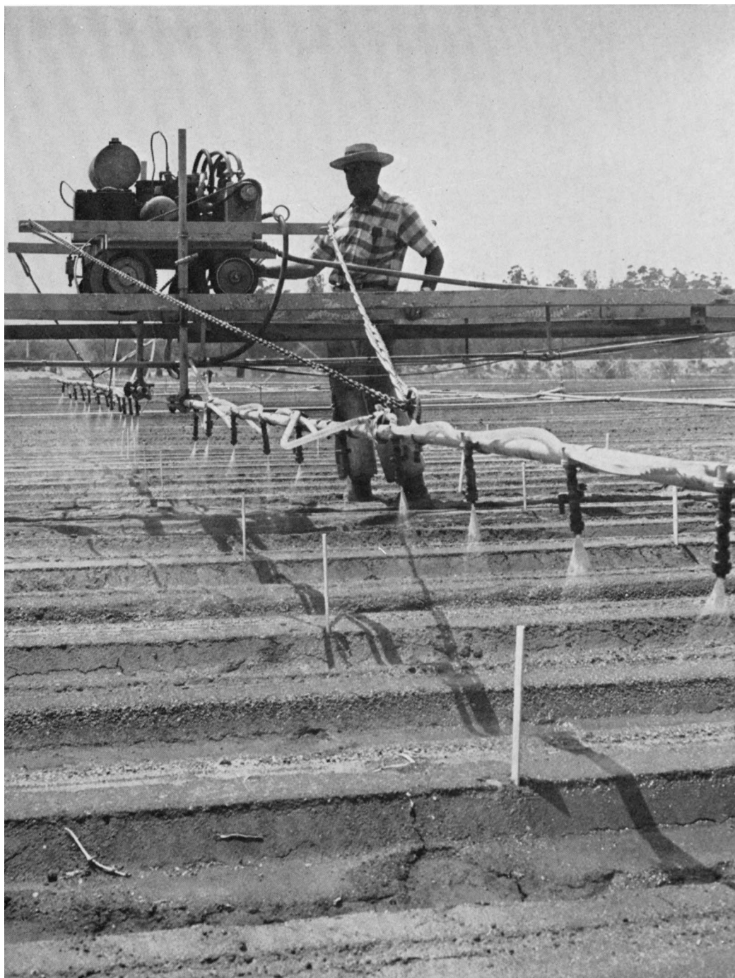
In studying effects of sprinkler irrigation on herbicidal activity, this precision irrigation test equipment was developed by University researchers (and manufactured by the Agricultural Manufacturing Co., Fresno) to allow accurate control of the amount and timing of precise amounts of overhead irrigation water.
