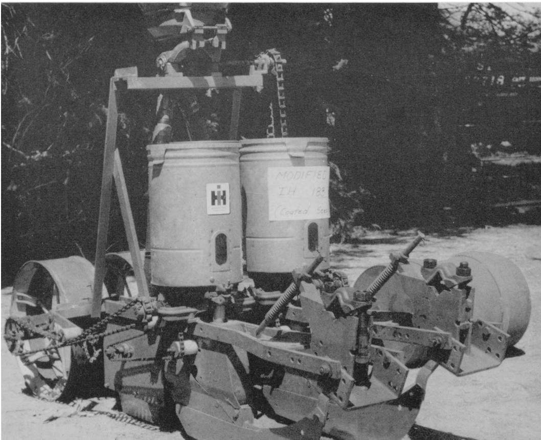
I.H.C. modified precision planter, as used in Salinas Valley lettuce test program with soil conditioners and herbicides.
