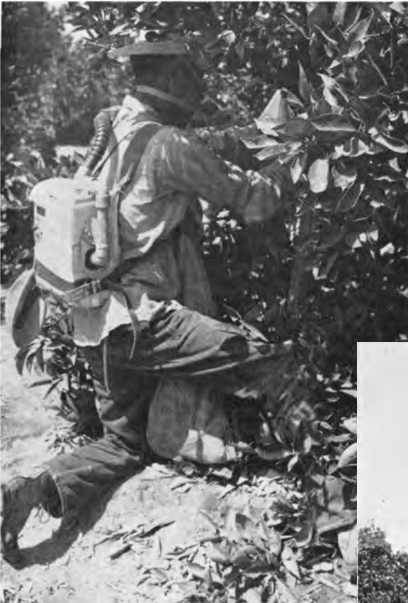
Picker shown with mask, respiration meter, and connecting hose as used during orange picking tests with fruit low on the tree in photo above, and from top of ladder in photo to right.
