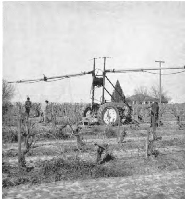
Two views of a tractor-mounted six-row pneumatic pruner working
