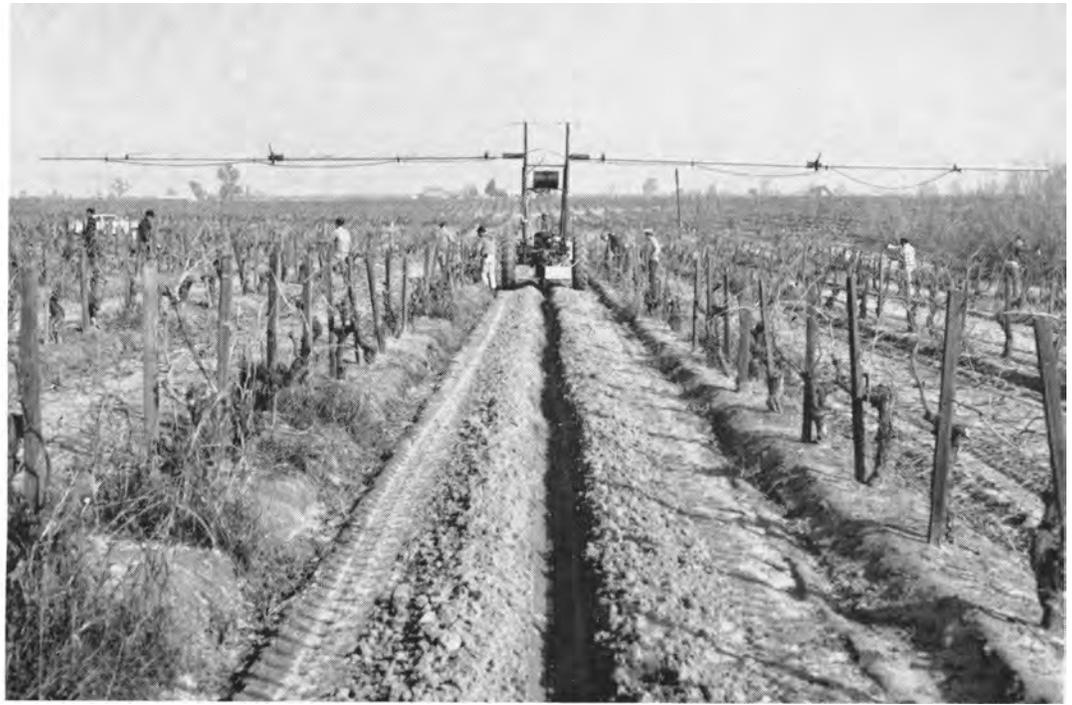
Fresno County raisin vineyard. The machine, provided with a creeper transmission and using the middle furrow as a guide, moves down the row unattended.
