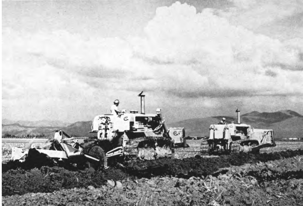
Rigolen plowing. A blade in front of the plow turns the surface soil into the bottom of the furrow to be covered by soil from below.
