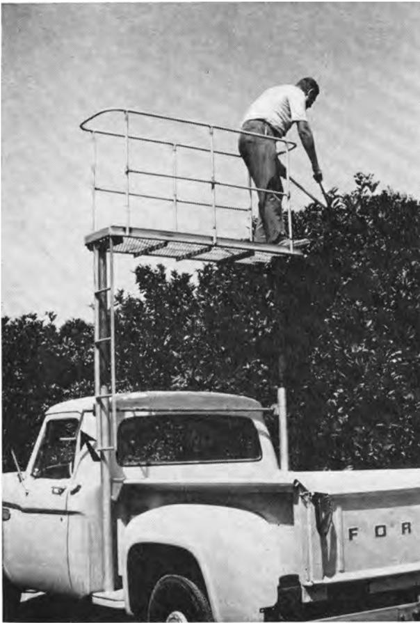
Photo left, elevated position for adjustable, truck-mounted platform showing a worker pruning a tree in a citrus orchard. Arrow points to crank used to wind cable within telescoping pipe supports.
