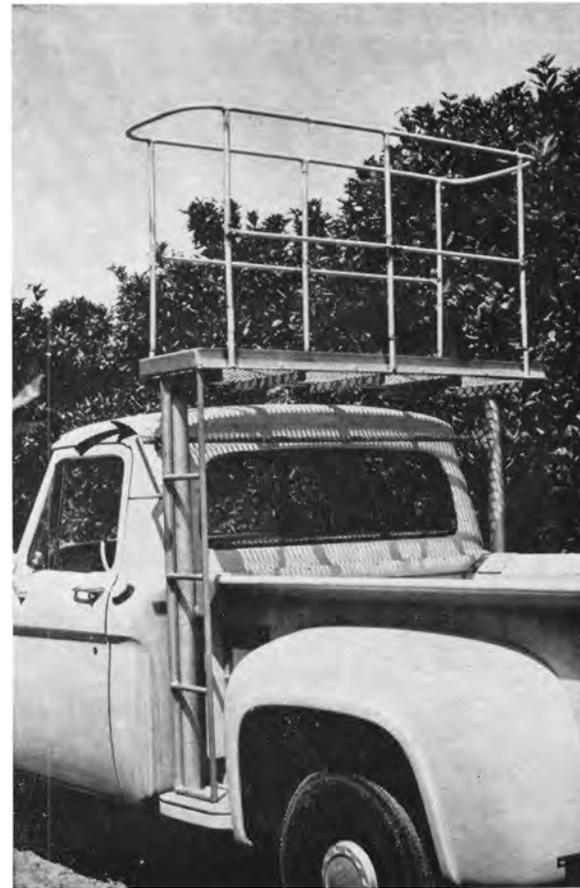
Photo right, shows down-position of the truck-mounted platform. Waist-high guard rail may be hinged to fold down, or made detachable to allow clearance and reduce wind resistance on the highway.
