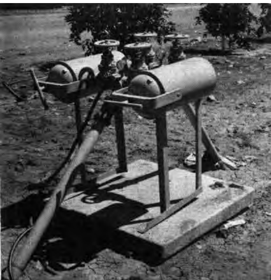
Two barrel-type filters mounted side by side. One is left in operation while the other is being cleaned.
