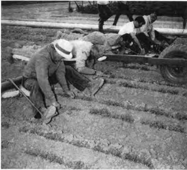
Figure 1. This experimental carrier provides three seated and three prone positions. Workers alternate at the end of each row.
