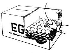
Egg with thermocouple wire for temperature measurement was placed near center of each case during the test procedure.
