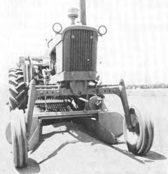
Front view of 1965 harvester with blade and front of conveyor at operating depth in sandy loam soil at Davis.
